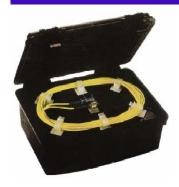
Mechanical and fusion splices- can be placed inside the test case for OTDR demonstration purposes. (Special Request)
